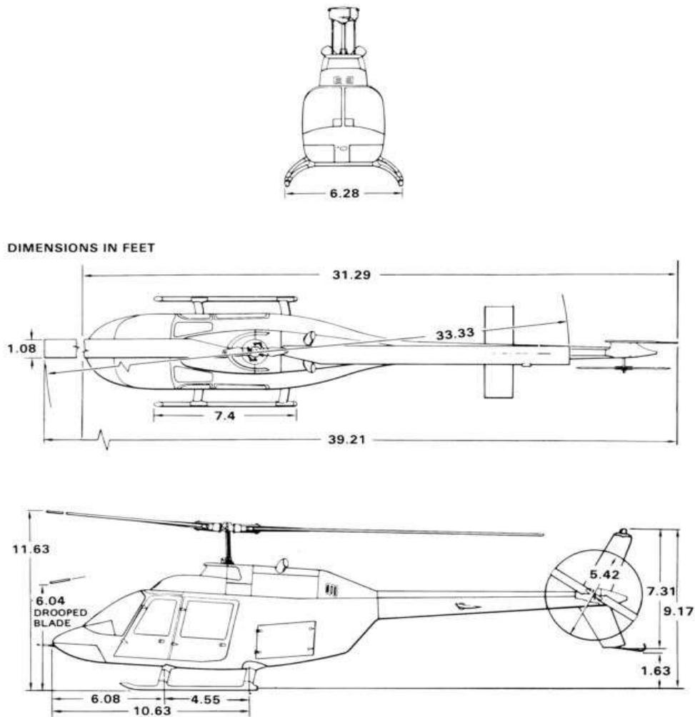
The main rotor assembly is a two-bladed, semi-rigid, see-saw type rotor with under slung mounting. The main rotor blades are all metal construction with an aluminium alloy honeycomb core, aluminium skins, spar and trailing edge strip. All the structural components are joined by means of metal-to-metal bonding.
