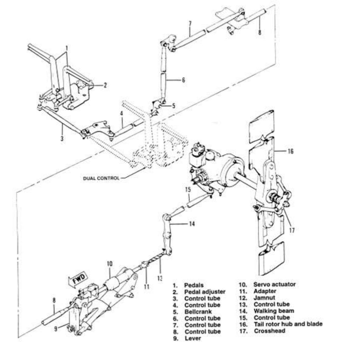
The tail rotor (anti-torque) control system includes control pedals, pedal adjuster, push-pull tubes, bell cranks, and a pitch control mechanism mounted through the tail rotor output shaft. Actuation of pedals causes pitch
